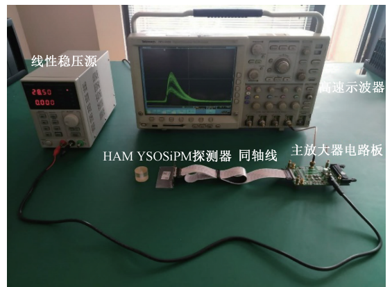
图 4 背散射探测器单一探测单元能量性能测定平台 Fig.4 Photo of the energy performance measurement platform of the single detection unit of backscattering detector
