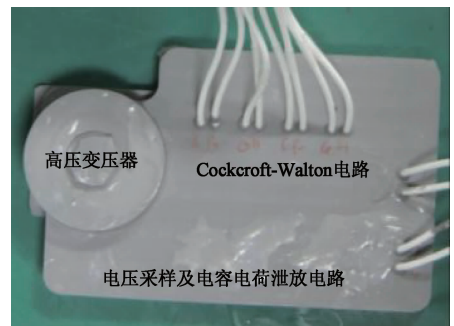
图11 高压组件灌封后实物 Fig.11 Photo of the encapsulated high voltage PCB assembly
