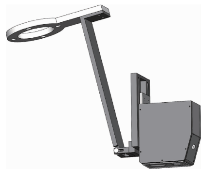
(b) 装配后线结构光传感器示意图 (b) Schematic diagram of the line structured light sensor after installation
