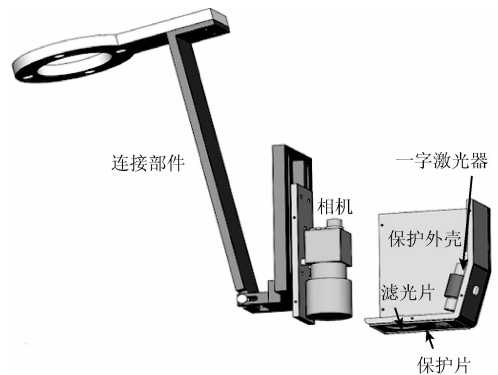
(a) 装配前线结构光传感器部件示意图 (a) Schematic diagram of the line structured light sensor before installation
