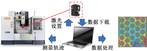
(c) 点云数据的获取 (c) Acquisition of point cloud data
