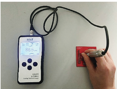
图 8 涂层测厚仪测量过程 Fig. 8 Coating thickness gauge measurement process
